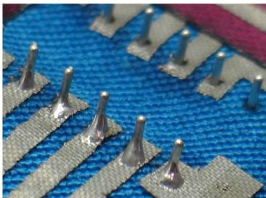
**Fig. 2** Solder joints on a fabric PCB
