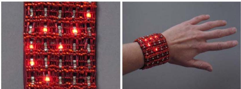
**Fig. 10** *Left* the first layer of the fabric PCB that powers the bracelet. *Right* a flat view of the bracelet
