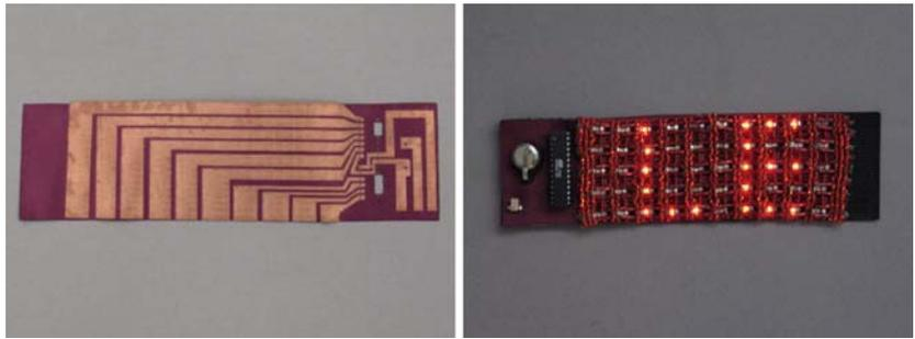
**Fig. 11** The socket button used to hold the microcontroller that powers the shirt shown in Fig. 3. *Left* Stitching the socket. *Right* The finished button
