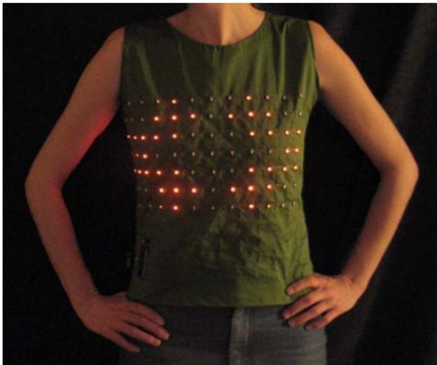
**Fig. 8** A wearable LED display matrix: a shirt embellished with LED sequins
